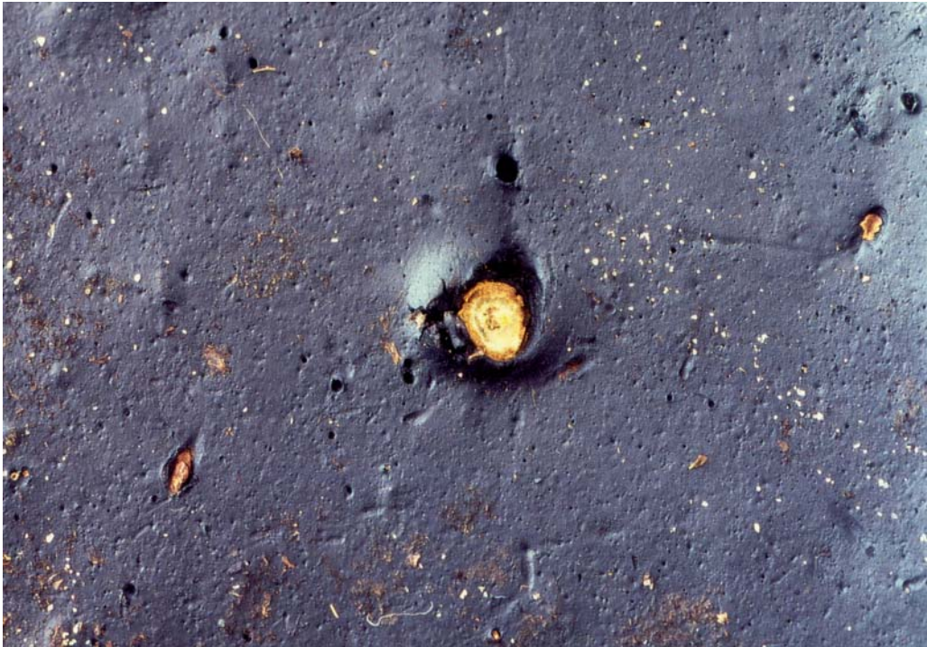
Figure 1: Sheet surface with root penetration
