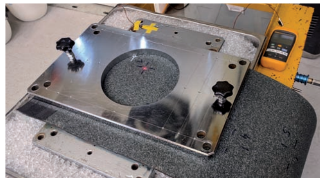
Test on rigid support according to VKF Test Protocol no. 09.
